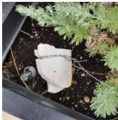
Photo 5. The mold with the wire binding it closed. Note the air vents are visible here.
