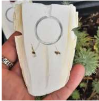
Photo 2. The cuttlebone mold. Note the distance from the top edge, the sprue, and the vent hold cut into the mold. The grooves for the binding wire are clearly visible along the sides.
