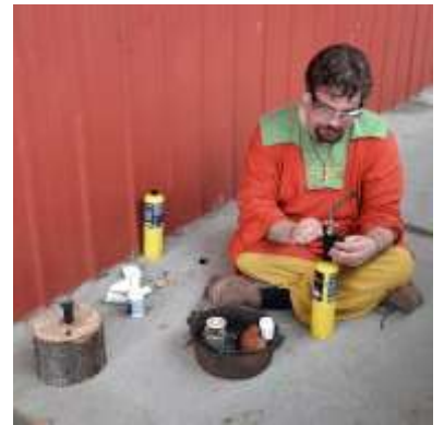
Photo 6. Preparing to cast a ring. The cast is securely wired closed and propped upright between the rock and the Dutch oven. The crucible of silver is to the left of the rock.
