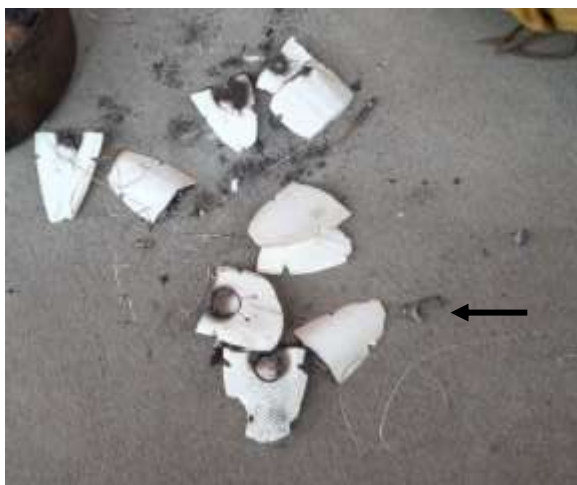
Photo 7. The results of the casting process. Note how the molds are scorched due to contact with the flame during pouring. The incomplete ring (arrow) was probably the result of inadequate venting and rapid solidification of the silver during the pour.
